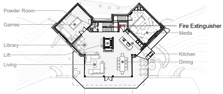
Level 3 - Extinguisher Plan
